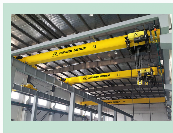
OVERHEAD CRANE 5 TAN
